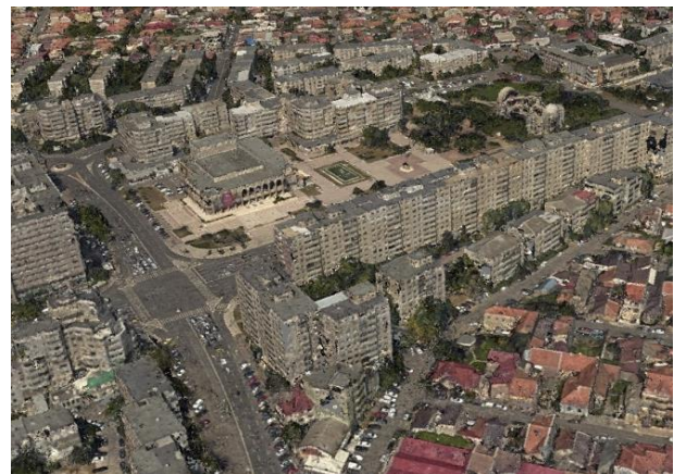
Figure 10. 3D model (point cloud) generated from the calibration mission data
