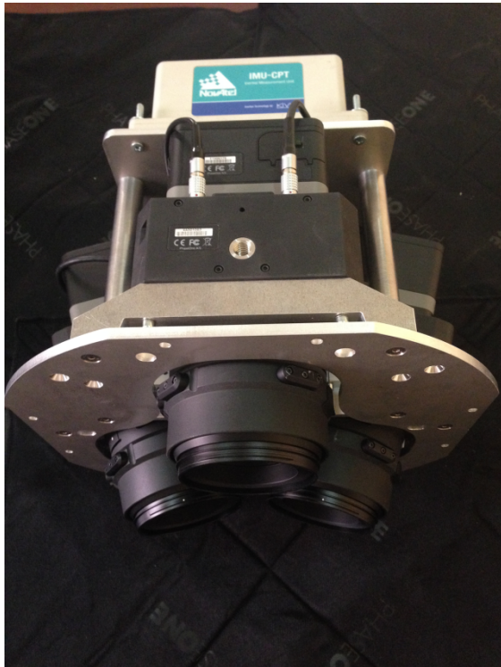
Figure 1: Camera head based on 3 midformat cameras to generate nadir and 2 oblique views
