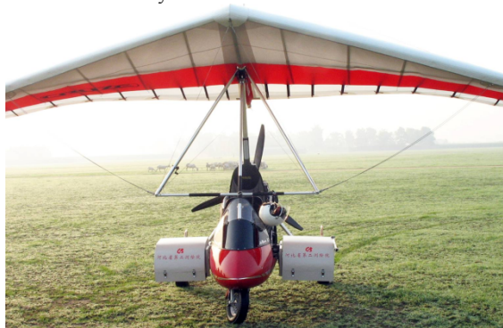
Figure 2. Microlighte-Trike as a platform for aerial surveying for monitoring earthquake disasters in China
